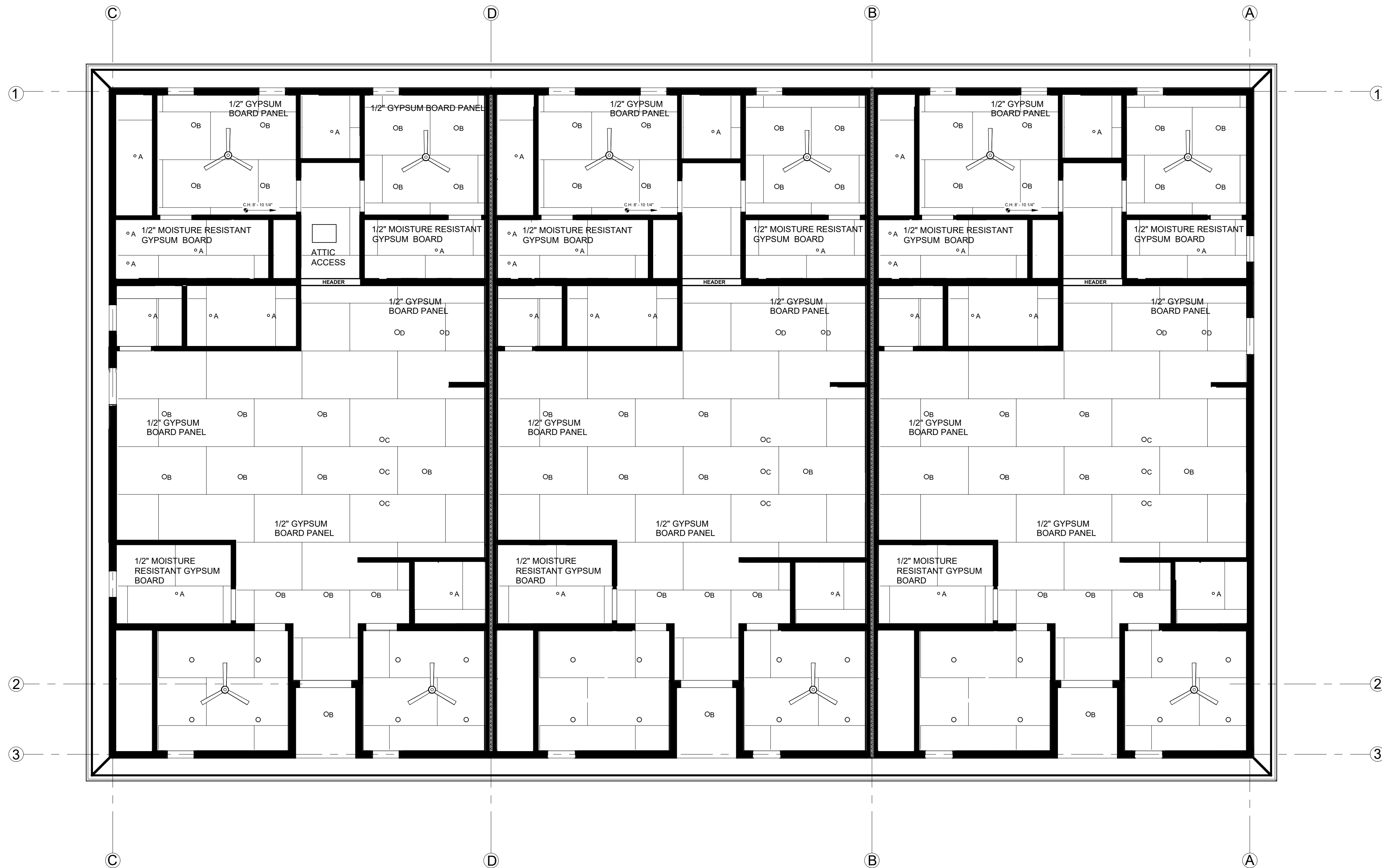
1 REFLECTED CEILING PLAN 3/16" = 1'-0"
